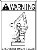
KEEP ATTACHMENT AWAY FROM CAB AND MACHINE. FAILURE TO DO SO MAY RESULT IN SEVERE INJURIES OR DEATH OR DAMAGE TO THE BOOMCYLINDER, HYDRAULIC HOSES OR THE CAB.
